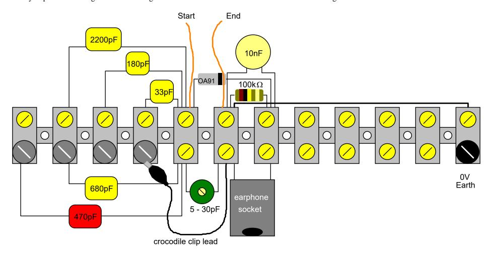
Connect a 9V battery to the RED and BLACK terminals on the diagram on page 3. Plug an input into the transmitter. This can be a microphone, guitar or output from an MP3 player but should give an output signal of at least 0.5V, or the modulation may be too weak to hear.
