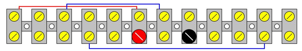
2). Take the three 2N3904 transistors. Carefully bend the leads so that they will fit as in the diagram below. Trim the leads if necessary. Ensure that they are fitted the correct way round.
