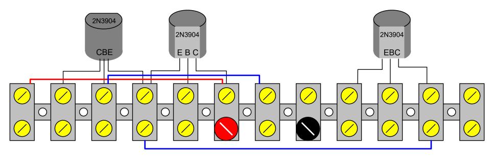
3). Take the four 10kΩ resistors (brown, black, orage, gold) and the 220Ω resistor (red, red, brown, gold). Add some insultaion to the lead of one of the 10kΩ resistors. Carefully bend the leads so that they will fit as in the diagram below. Trim the leads if necessary. It does not matter which way round they are connected.
