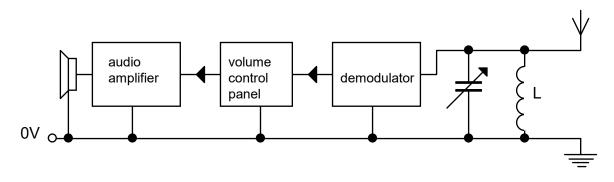
The tuning capacitor, inductor, aerial and earth are connected to the demodulator.
