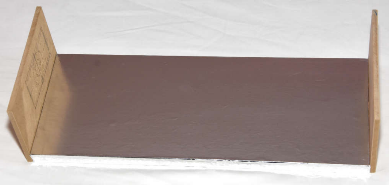
Baseboard covered in aluminium foil with end panels attached and showing the foil extending down the sides of the baseboard.
